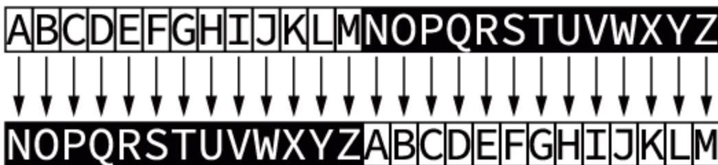
Figure 4.5 The rot13 filter swaps the upper half of the alphabet with the lower half, effectively "rotating" the characters by 13 positions.
